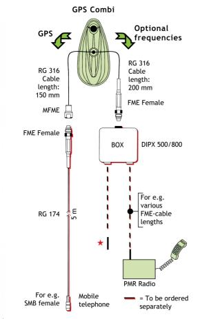
★ FME-Connector suitable for Mobile telephone in question.
